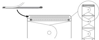
2 Assemble the Foldio by the magnets / Attach the holder to the top of the rear inside of the Foldio to fix the backdrop.
